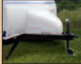
Molded bottle cover protects the LP bottles and battery
