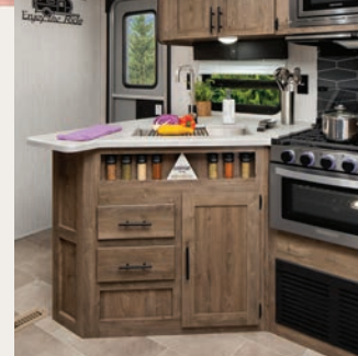
L-shaped galley features a single bowl sink, high rise faucet, sink cover and seamless countertops. Access storage cabinets from both front and back sides
