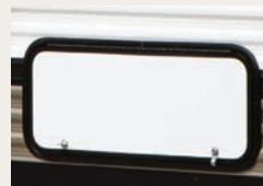
Radius compartment doors are silicone sealed to protect from the elements
