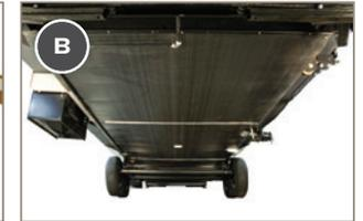
**B** 5/8" tongue and groove plywood glued and screwed to aluminum framing.
