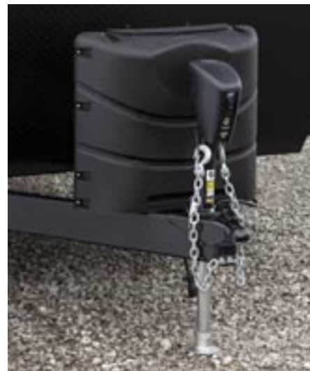
(2) 20 Lb. LP bottles with cover, manual jack with chain hooks - standard (Power Stance tongue jack, auxiliary cord - optional)
