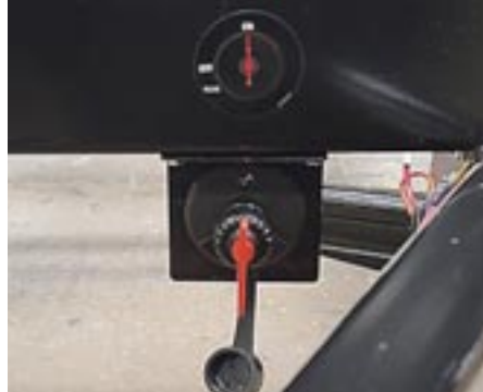
Seafo battery isolator switch prevents power drain. Operates by removable key.
